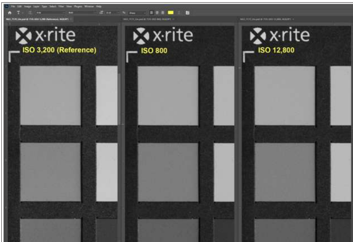
Picture 8: Screenshot showing (at 100%) the three images taken at three different ISO values.
